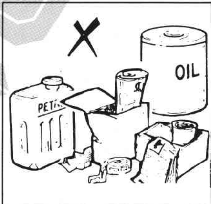
Before commencing cutting, clear the area of flammable materials.
