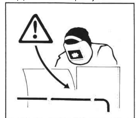
Check for 'hidden' wires before cutting
